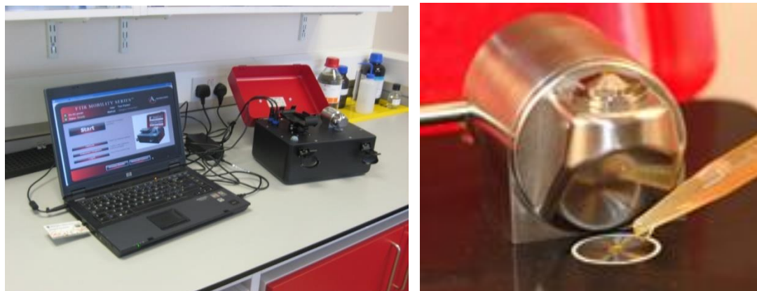
Fig. 7. Agilent 4500 Series Tumbler-IR portable FTIR spectrometer. The photo on the right shows a close-up of the head in the position for applying the sample to the window
