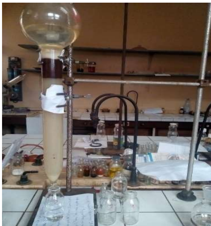
Figure 3.3: Column chromatography protocol and set up
